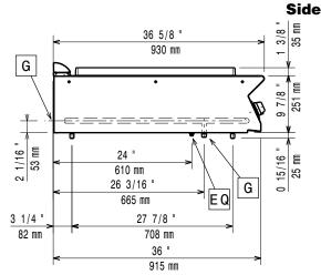
EQ = Equipotential screwG = Gas connection
